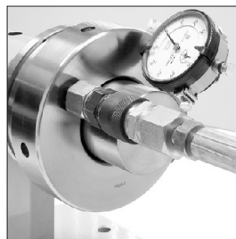
6 | Insert the high pressure hose to the hydraulic nut to start gap reduction of the bearing according to size of bearing
